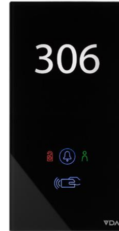
RFID 13.56 mhz Reader + Room Number
